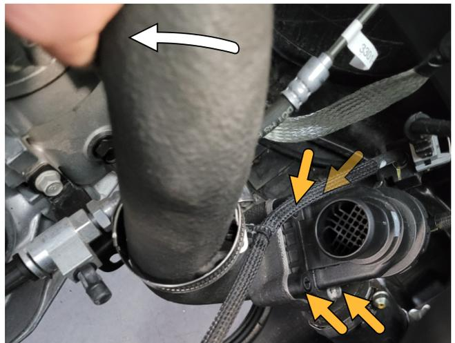
6) Install the GFB valve using the supplied screws. A 5mm T-handle hex key helps with the rear screws:
