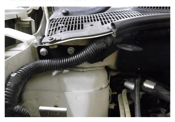
8. Re fit the brake fluid reservoir, just slide it back into place.
