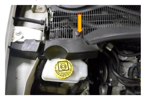
5. Using a flat blade screwdriver push the retaining clip inwards while holding the brake fluid reservoir, then slide it out to the righthand side. (If you have a LHD vehicle you can skip this step.)
