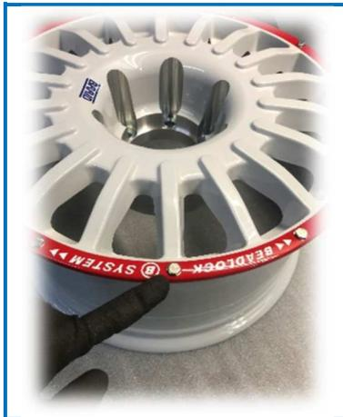
1. To mount the tyre all tapered 45 degrees screws must be previously removed.
