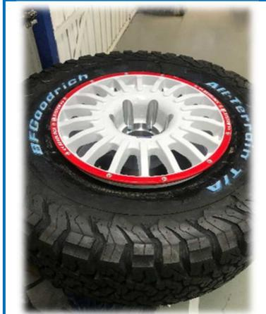
2. Then, the tyre can be mounted in its usual way. Once the tyre is inflated, with higher pressure than standard, we must tighten the tapered screws until they collide against the wheel. Only after all the screws are screwed in, we can proceed to restore the normal tyre pressure.
