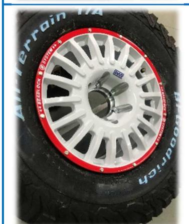
3. The screws have a special sealing gasket washer. It is essential to keep these washers pressing the rim flange. Otherwise, the screw would be stuck more than expected in the tire and the inflation pressure would be lost in the case of mounting without a camera.
